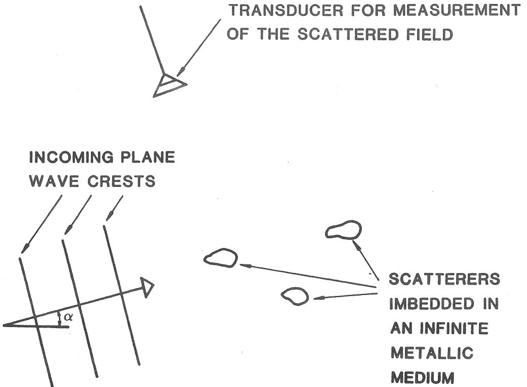
**Figure 2.** The idealised set-up. Plane waves moving in the direction  $\alpha$  impinge on the inclusion(s). The scattered ultrasonic field  $|u_s|$  is detected by a movable transducer. The incident ultrasound could be replaced by a conical beam without loss of generality.
