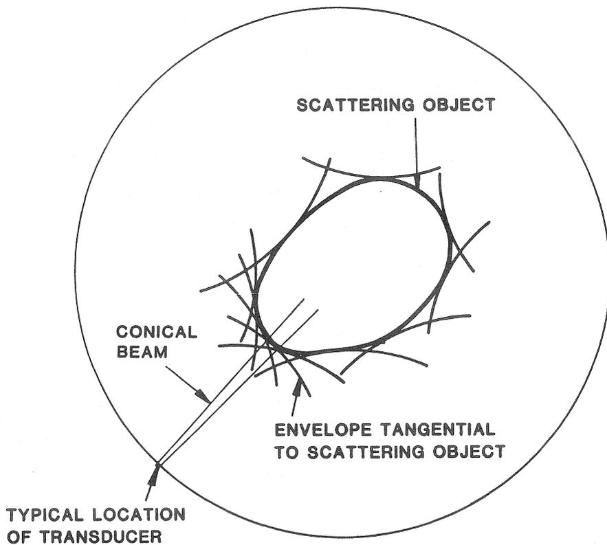
**Figure 10.** Illustration of an arrival time envelope calculation. The scattering object lies within the envelope of exclusion; as many locations as desired may be taken for the transducer.
