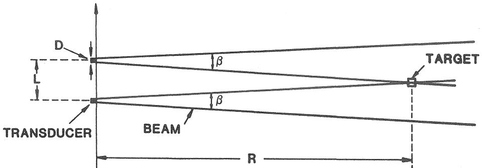
Figure 6. The synthetic aperture method. The actual aperture of the transducer is  $D$  and the synthetic aperture is  $L$ .
