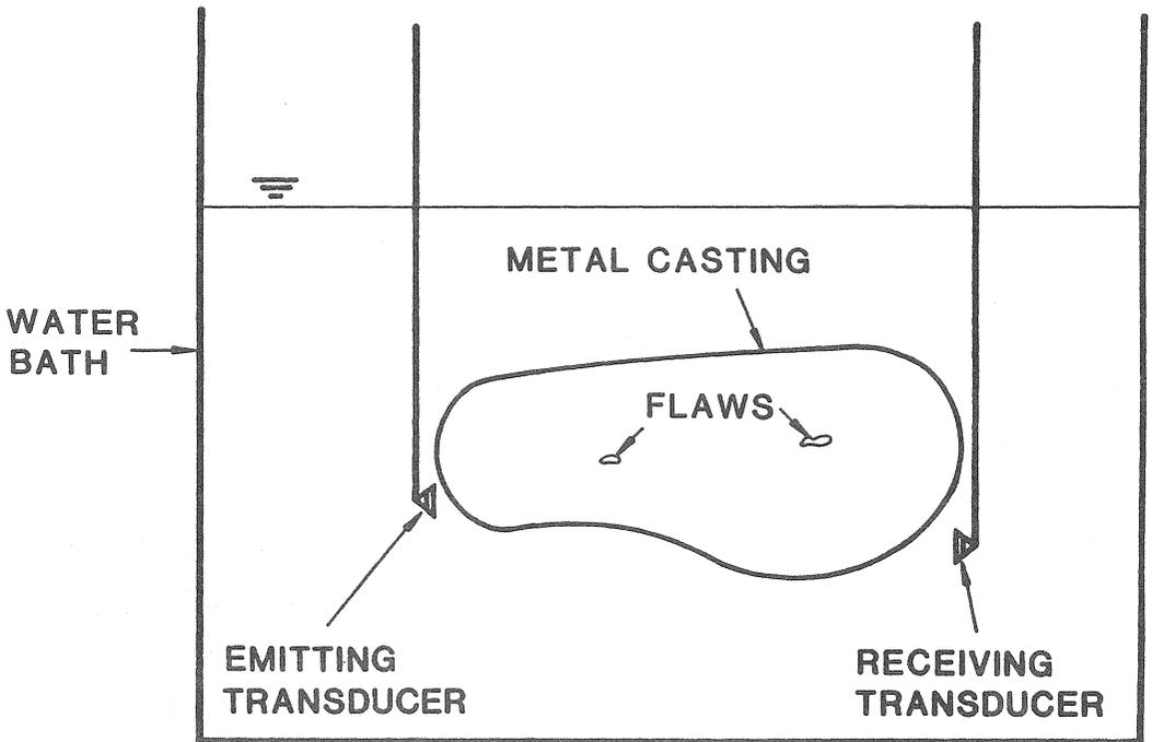
Figure 1. Illustration of the present experimental set-up. Both transducers are movable.
