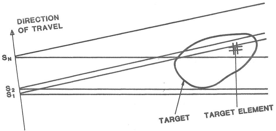
Figure 7. Illustration of transducer locations  $S_1, S_2, \dots, S_N$  and the target element.
