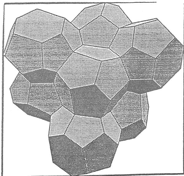
**Figure 13.13.2.** The relaxed stacked tetrakaidecahedra and occasional dodecahedra of Weaire and Phelan beat Kelvin's conjecture by about 0.3%. Graphics by Ken Brakke on the Brakke Evolver from Brakke's early Geometry Center report.
