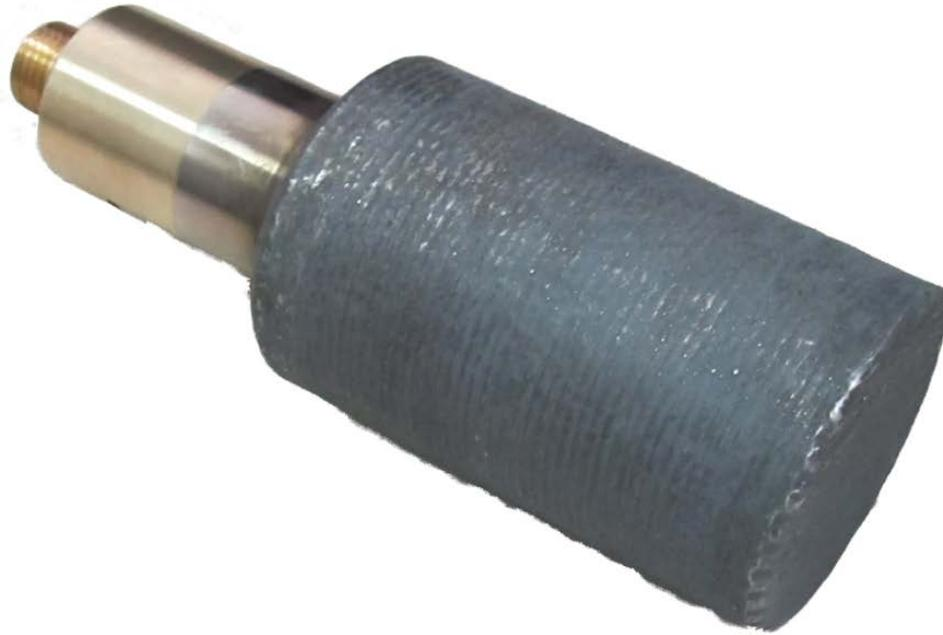
CNT cathode surface through laser cladding can generate field enhanced EEE and surface-flashover EEE.
