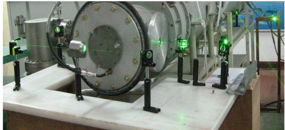
A Mach-Zehnder interferometer was designed and used to measure the plasma density in the diode.
