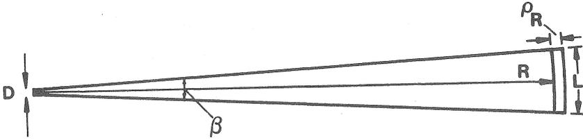
Figure 5. Illustration of the radial and azimuthal resolutions of a pulsed beam. The length of the pulse is  $\tau$ , so that the radial resolution is  $\rho_R = \frac{1}{2} c \tau$  where  $c$  is the speed of ultrasound in the medium. The reflected signal could come from the near edge of the zone of resolution and occur at the start of the pulse, or from the far edge at the end of the pulse. The azimuthal resolution is  $\rho_A = L$ .
