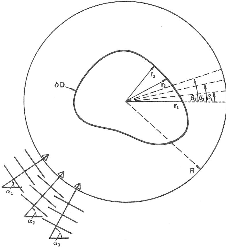
**Figure 4.** Illustration of a hypothetical inverse problem. The total scattered field is measured at stations  $\beta_1, \beta_2, \dots, \beta_M$  at radius  $r = R$ . The incident ultrasonic plane waves are propagating in one of the directions  $\alpha_1, \alpha_2, \dots, \alpha_L$ ; and it is required to determine the unknown coefficients  $r_1, r_2, \dots, r_N$  by minimizing  $E$  as defined in equation (3.5).
