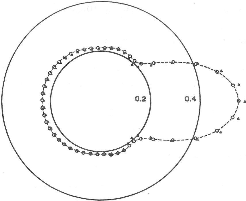
**Figure 3.** A polar plot of the magnitude  $|u_s|$  of the scattered field at radius 10 produced by a plane ultrasound wave impinging on a circular cylinder of radius 1. The incident beam is from the left and the wavenumber  $k$  is 3. The dashed line shows the separable solution (3.4), the open circles show the full solution (3.2) whilst the open triangles show the leading far-field approximation to (3.2).
