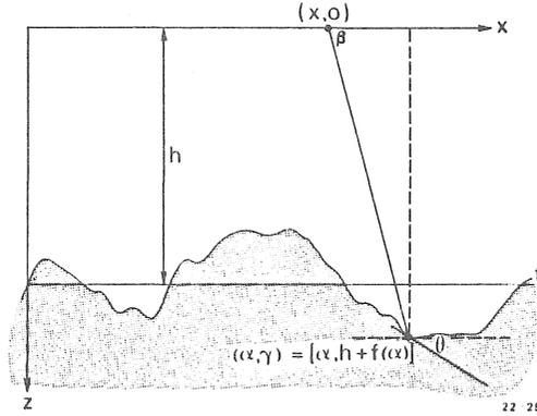
Figure 3. The co-ordinate system used in the derivation of the simplified two-dimensional relief equation.
