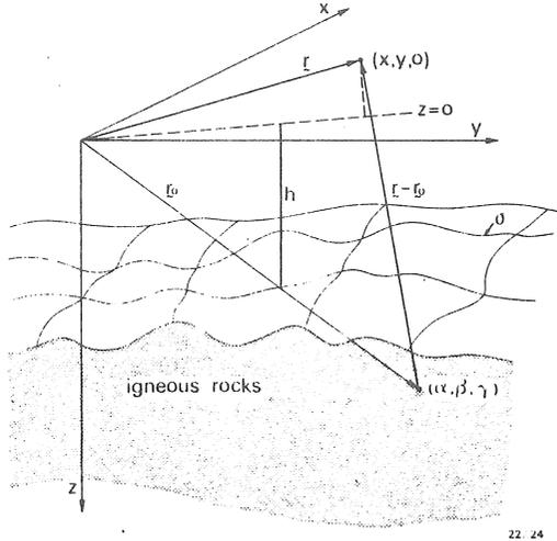
Figure 2. The co-ordinate system used in the derivation of the full three-dimensional relief equation.
