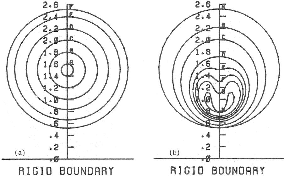
Figure 1. Bubble shapes for  $\gamma = 1.5$  during (a) expansion phase at dimensionless times A) 0.001553 B) 0.024138 C) 0.090953 D) 0.214281 E) 0.466561 F) 0.973926 and (b) collapse phase at dimensionless times A) 0.973926 B) 1.729799 C) 1.881328 D) 1.988787 E) 2.024132 F) 2.044900 G) 2.063839 H) 2.093078.
