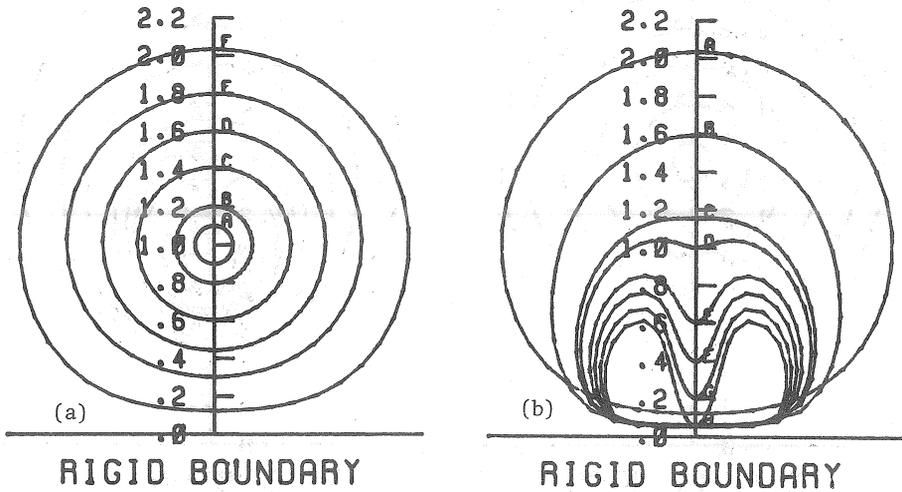
Figure 2. Bubble shapes for  $\gamma = 1.0$  during (a) expansion phase at dimensionless times A) 0.001553 B) 0.009084 C) 0.053140 D) 0.142416 E) 0.312960 F) 0.975561 and (b) collapse phase at dimensionless times A) 0.975561 B) 1.849750 C) 2.023160 D) 2.048726 E) 2.097308 F) 2.121807 G) 2.144854 H) 2.162422.
