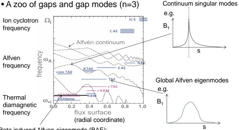
Beta induced Alfven eigenmode (BAE): Low frequency mode that exists due to finite beta (pressure)
