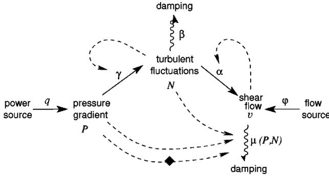
FIG. 1. A plasma turbulence governor, showing the coupled rates and feedback processes that contribute to the dynamics of  $L$ - $H$  transitions. Solid arrows indicate generation rates, wavy arrows dissipation, dashed arrows feedback on rate coefficients; the black diamond indicates negative feedback.
