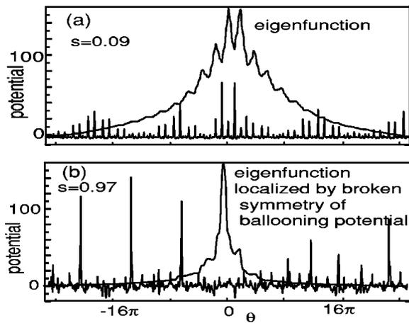
FIG. 7. The localization of the ballooning mode eigenfunction for 4.3%  $\beta$  and the ballooning potentials on flux surfaces near the magnetic axis and the plasma edge. The eigenfunctions are normalized to the same maximum value. The ballooning potential is increasingly aperiodic far from the magnetic axis, where axial symmetry is more strongly broken.
