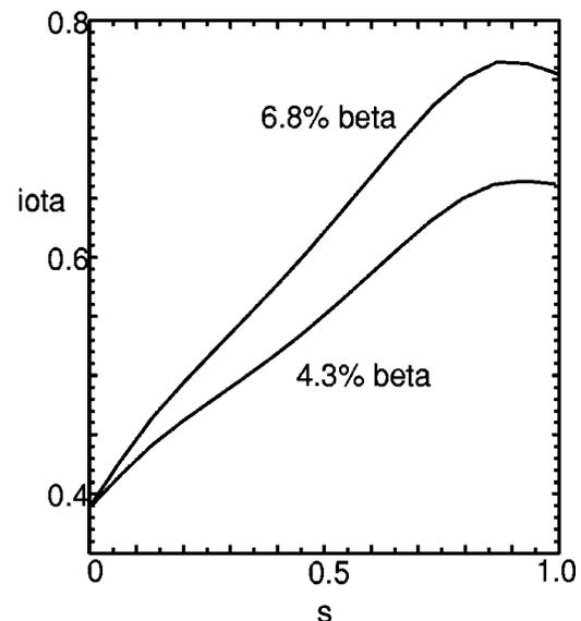
FIG. 3. Iota profiles of two ballooning unstable equilibria of the QAS. Higher pressure drives bootstrap currents which increases the field line transform iota at 6.8% compared to 4.3%  $\beta$ .
