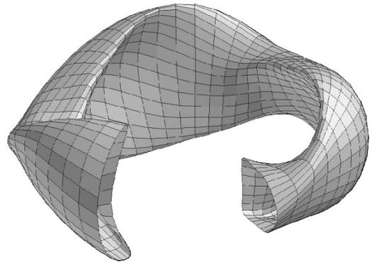
FIG. 1. The outermost flux surface of the three field period quasiaxially symmetric stellarator.
