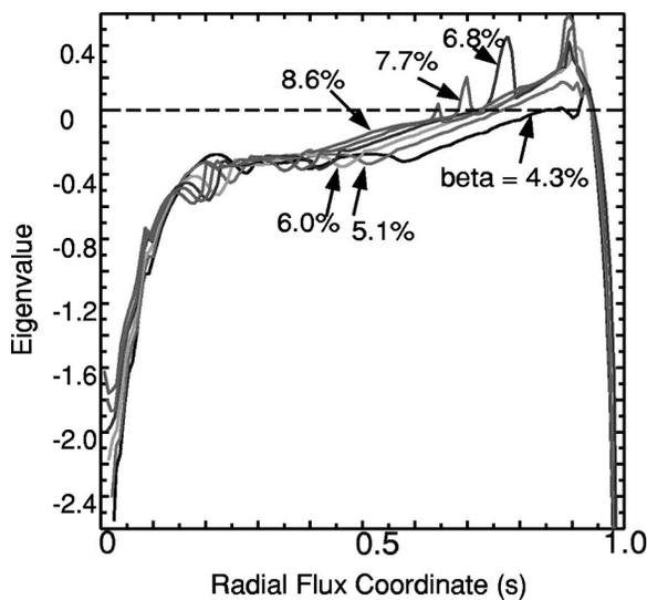
FIG. 4. Ballooning eigenvalues as a function of the radial coordinate for a  $\beta$  scan above the ballooning limit of QAS3\_LI383. 129 radial flux surfaces are used. Singular points occur where rational values of  $q$  are found and for locations of very low shear.
