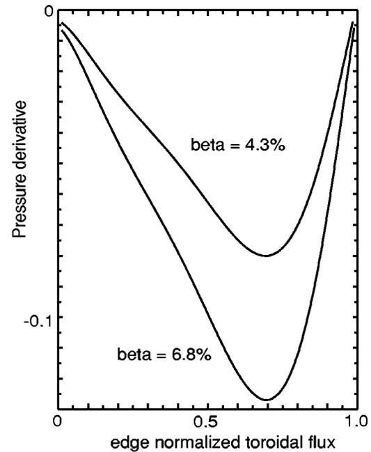
FIG. 2. Derivatives of the pressure profile for two ballooning unstable equilibria of the QAS, obtained with fixed boundary VMEC. Steeper pressure results in higher  $\beta$ , but also drives MHD instability.
