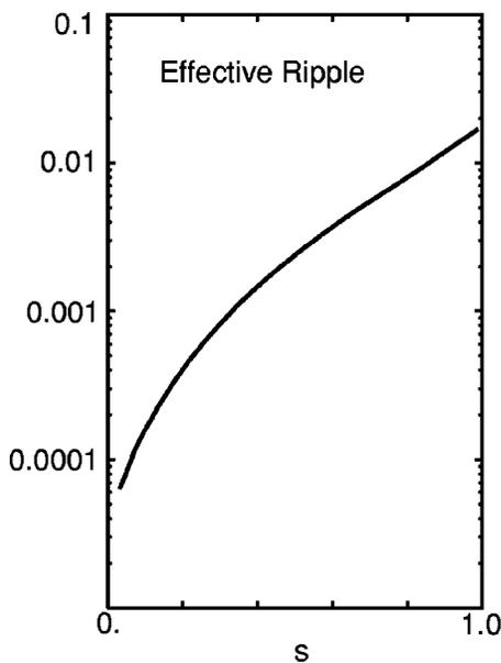
FIG. 8. Effective field line ripple for the QAS at 4.3%  $\beta$ .
