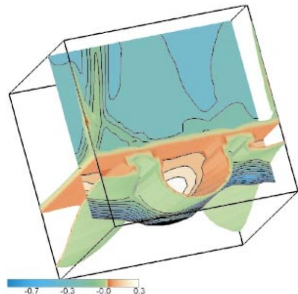
FIG. 6. (Color) Ballooning spectrum of 4.3%  $\beta$  QAS configuration: the marginal isosurface at  $\lambda(s, \alpha, \theta_k) = 0$ , for the same color map and reduced 3-space as in Fig. 5. Also shown is the  $(s, \alpha)$  plane at  $\theta_k = 2\pi/3$ .
