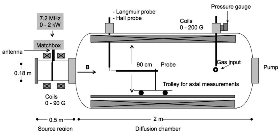
FIG. 1. A schematic of the WOMBAT (waves on magnetized beams and turbulence) plasma experiment.<sup>36</sup>
